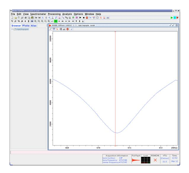
5. Acquire and process the 19F experiment using the commands: rga, zg, ef, apk, abs n
