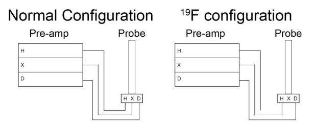
4. Type "wobb" at Topspin command line. Go to the probe. You'll have to tune the probe to 19F by turning the silver screw labeled "T" ~four turns **to the right**. If you have it tuned correctly it should look like the following:
